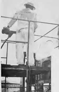
A ROSS carrier gets a thorough steam cleaning first before it is given its monthly maintenance which includes a grease job, oil change and tune-up.
